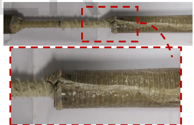
Figure 10: Failure Mode of G12-NW-16.25 (Sleeve Cracking)
