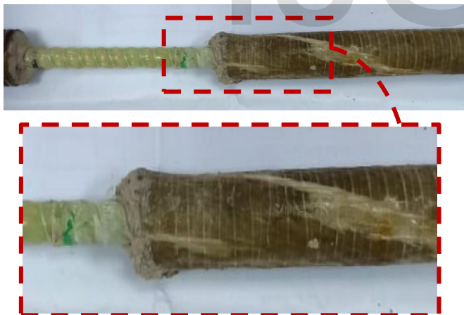
Figure 9: Failure Mode of G12-NW-13.75 (Sleeve Cracking)
