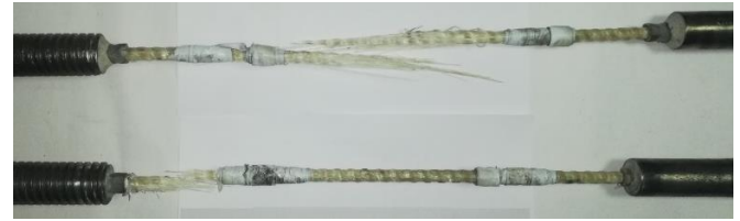
Figure 7: GFRP Bars Tensile Failure
