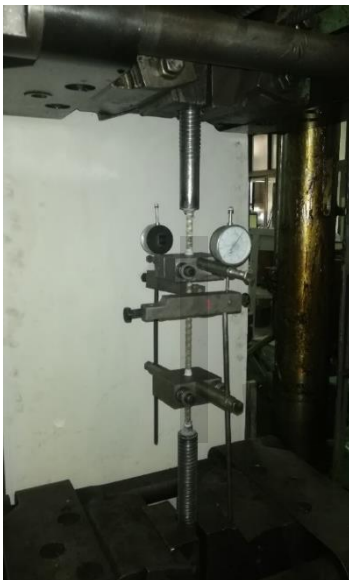
Figure 4: Test Setup for Control Specimens Tensile Test
